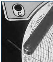
Chart recorder stylus and time line groove
