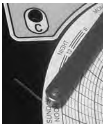
Chart recorder stylus and time line groove
