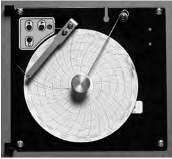
Chart Recorder with paper installed
