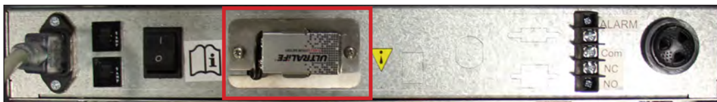
Monitoring system backup battery
