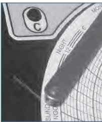
Chart recorder stylus and time line groove
