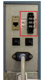
Remote alarm interface.
