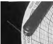
Chart recorder stylus and time line groove
