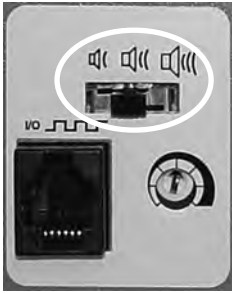
Alarm volume control (circled).
