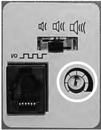
Alarm delay control (circled).
