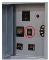
*i.C*<sup>3</sup> Monitoring System / Access Control backup battery ON/OFF switch (circled)
