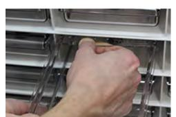
Tab on outer edge engaged with slot
