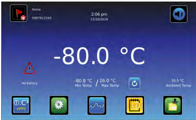
Home screen with active alarm
