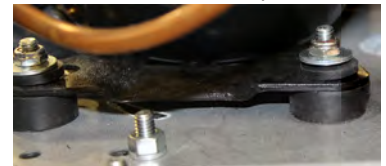
Rubber foot installed
