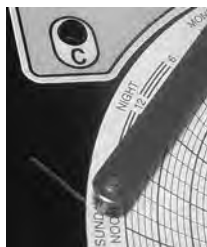
Chart recorder stylus and time line groove
