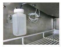
Left: Probe bottle with temperature probe
