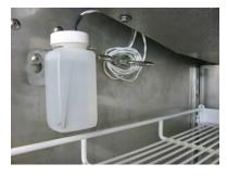
Left: Probe bottle with temperature probe
