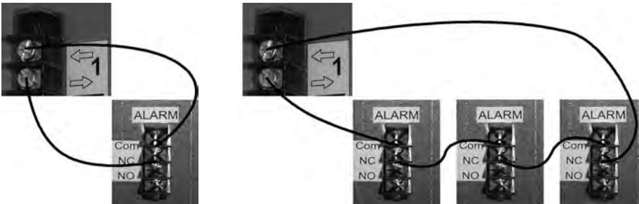
Zone connections for a normally-closed configuration. Left: One device. Right: Multiple devices.
