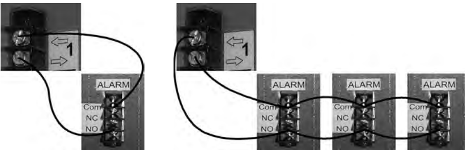
Zone connections for a normally-open configuration. Left: One device. Right: Multiple devices.
