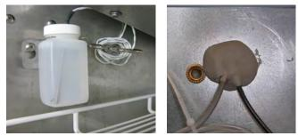
Left: Probe bottle with temperature probe. Right: Access port on rear of freezer.
