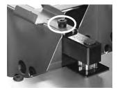
Basket installed on lift-out arm. Finger knob circled.
