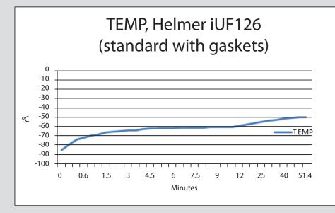
The time for the average cabinet temperature to reach -50°C with the outer door and top inner door open was 51.4 minutes.
