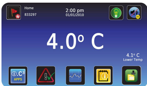
Home screen - alarm muted
