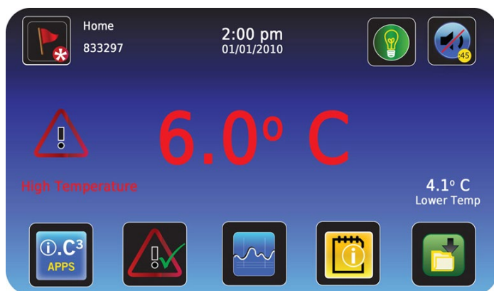
Home screen with active alarm
