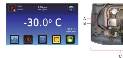
Left: Front view, LCD touchscreen. Right: Rear view of display, showing display board.
