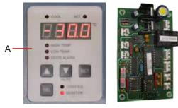
Left: Horizon display with touchpad. Right: Rear view of display showing monitor/control board.
