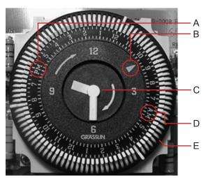
Horizon Series defrost controller with current time set to approximately 9:30 PM.
