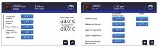
Left: Temperature Controller Programs screen. Right: Temperature Calibration screen.
