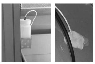
Left: Probe bottle with temperature probe. Right: Access port as seen from top of freezer.
