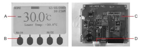
Left: Display assembly showing LCD and touchpad. Right: Display board.
