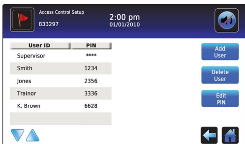
Access Control Setup screen
