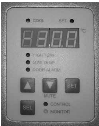
Horizon Series monitoring and control interface.
