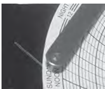
Chart recorder stylus and time line groove
