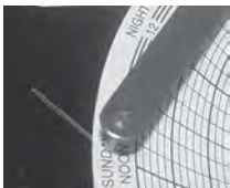
Chart recorder stylus and time line groove
