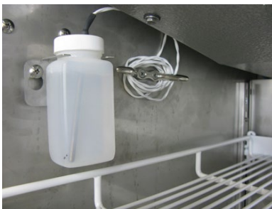
Probe bottle with temperature probe.
