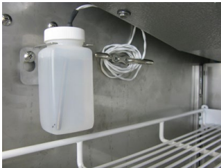
Left: Probe bottle with temperature probe. Right: Rear access port.
