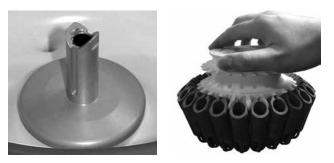
Left: Rotor shaft with alignment slot visible. Right: Grasping the rotor on the grip area.
