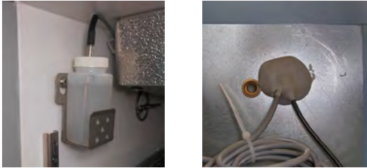
Left: Probe bottle with temperature probe. Right: Rear access port.
