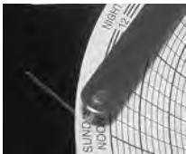
Chart recorder stylus and time line groove
