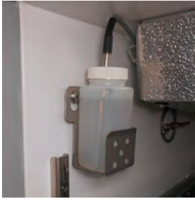
Left: Probe bottle with temperature probe. Right: Rear access port.
