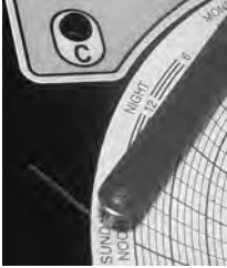
Chart recorder stylus and time line groove
