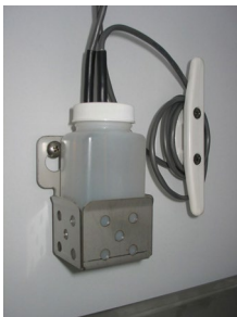
Left: Probe bottle with temperature and chart recorder probes.
