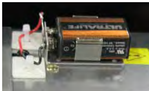
Monitoring system backup battery.
