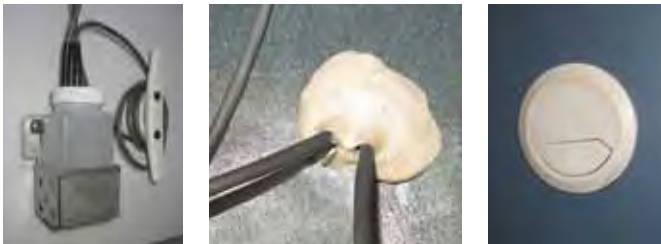
Left: Probe bottle with temperature and chart recorder probes. Middle: Access port as seen from the top of the refrigerator. Right: Access port on side of refrigerator. The number and location of ports varies by model.
