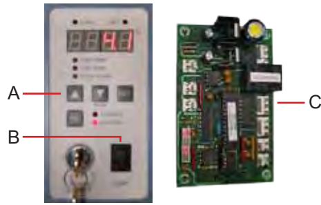
Left: Front view, Horizon touchpad. Right: Rear view of display, showing monitor/control board.
