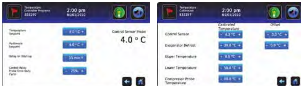
Left: Temperature Controller Programs screen. Right: Temperature Calibration screen.
