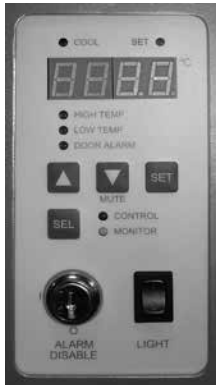
Horizon Series monitoring and control interface.
