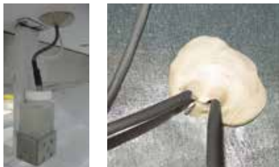
Left: Probe bottle with temperature probe. Right: Access port as seen from top of refrigerator.
