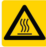
Caution, hot surface
