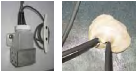
Left: Probe bottle with temperature and chart recorder probes. Right: Access port on top of the refrigerator. The number and location of ports varies by model.
