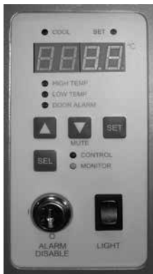
Horizon Series monitoring and control interface.
