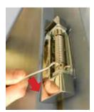
Rotate the spring using a J-hook tool then insert pin (left-hinged door shown).
