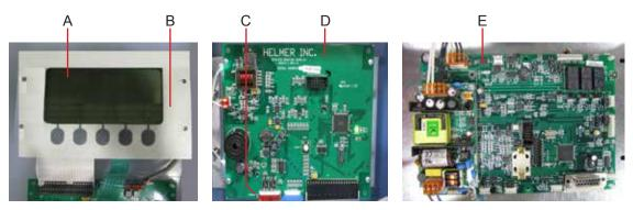
Left: Display assembly including LCD display and touchpad. Middle: Display board. Right: Control board.
