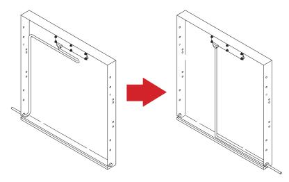
Left: Original cable routing (right-hinged door). Right: New cable routing (left-hinged door).
